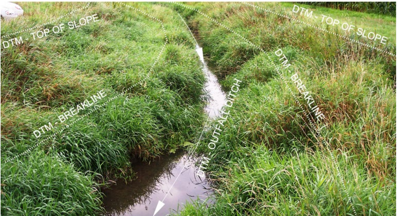
Figure 42 Example Outfall Ditch Survey
