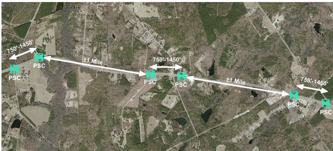
Figure 16 Primary Survey Control Layout
