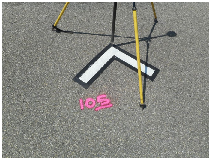
Figure 6 Example Mobile Lidar Ground Control Point
