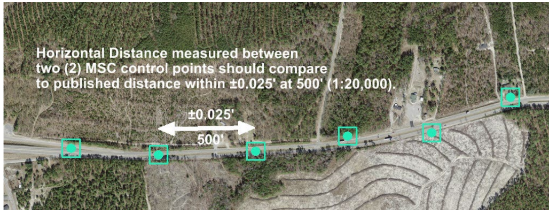
Figure 18 Horizontal Unadjusted Ratio of Precision
